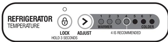
**NOTE:** You can lock the controls so the settings cannot be changed.
